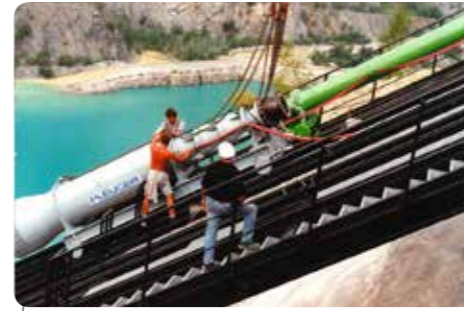
Wülfrath, Germany: Inclined installation of our submersible pumps, used for limestone mining.
